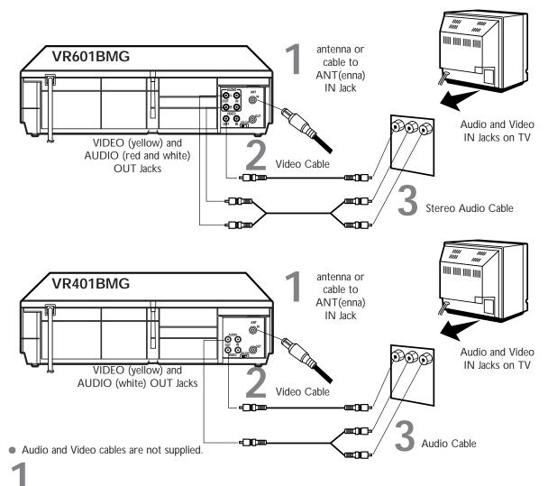
Connect the antenna or cable to the ANT(enna) IN Jack on the back of the VCR.
